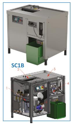
The machine is equipped with a passive safety system, guaranteed by the particular design of the intake hopper which prevents the access to the moving parts of the disposer while in use, and an active safety device which stops the disposer in case of accidental opening of the cabinet's lid. Permanent magnets are installed under the hopper to capture metals avoiding the risk of their accidental falling inside the disposer.
